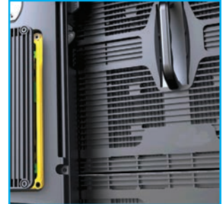
Each module is integrated with a dissipating plate for releasing heat with no fans
